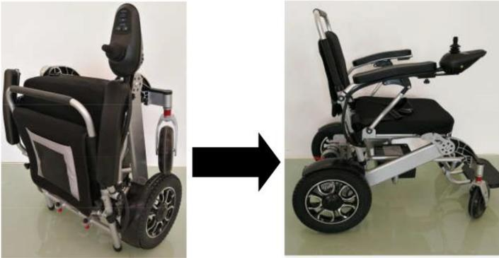
3. Lock Frame open with fold latch by flipping the wire loop up and securing.
