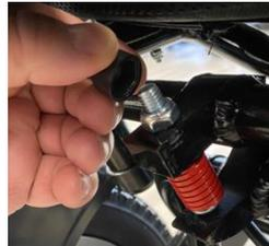
4. Lower the armrest and lock in place by turning the locking lever upwards.
