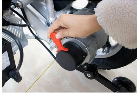
Note: The handle must be pulled up in the electric mode, otherwise the controller will give an alarm and cannot start. In manual mode, the power supply should be turned off, otherwise the push resistance will be very large.
