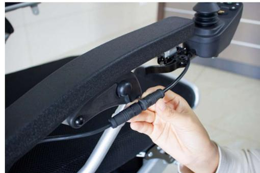
**Note:** When connecting the plug, it must be inserted in alignment with the notch, otherwise the plug insertion pin can be bent and damaged and cannot be used!
