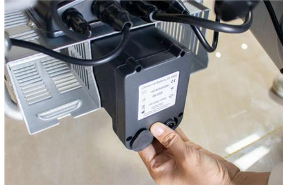
If the battery capacity needs to be increased, batteries with the same capacity can be connected in parallel. As shown in Figure. 9, there are two socket holes on the battery that can be inserted into either of them in parallel to increase the capacity.
