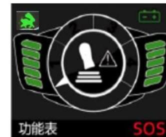
Joystick Failure: The center icon displays joystick malfunction.
