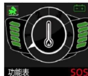
Overheat: The internal temperature of the driver or controller is too high, which may cause a malfunction and the wheelchair may not work properly.
