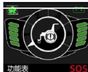
Left-side Motor Fault: Unable to communicate with the left wheel drive; Left-side motor is broken.
