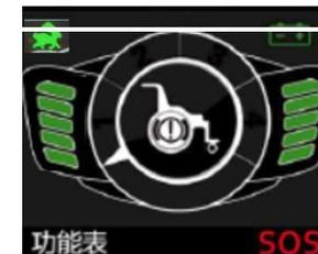
Right-side Motor Fault: Unable to communicate with the right wheel drive; Right-side motor is broken.
